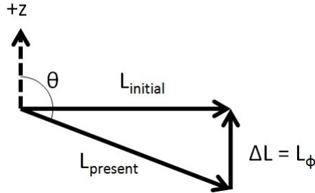
Figure 6: An angular momentum component in the z direction emerges as the gyroscope tips downward
