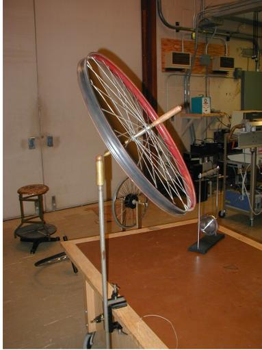
Figure 1: Bicycle wheel gyroscope demonstration used at the University of Rochester. Image credit: Thang V. Nguyen[6]
