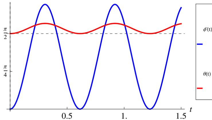
Figure 7: An angular momentum component in the z direction emerges as the gyroscope tips downward
