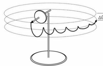
Figure 2: A precessing and nutating gyroscope. Image credit: Svilen Kostov and Daniel Hammer [5]
