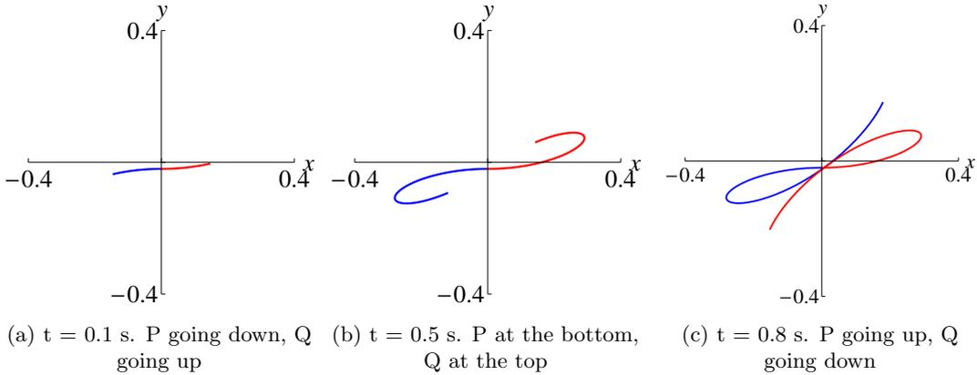
Figure 8: Trajectories of two points on the wheel. Point P (blue) begins on the top of the wheel, while point Q (red) starts at the bottom.
