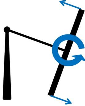
Figure 9: The forces required to alter the trajectories of the points on the wheel exert a torque about the axis, supporting it against the torque of gravity
