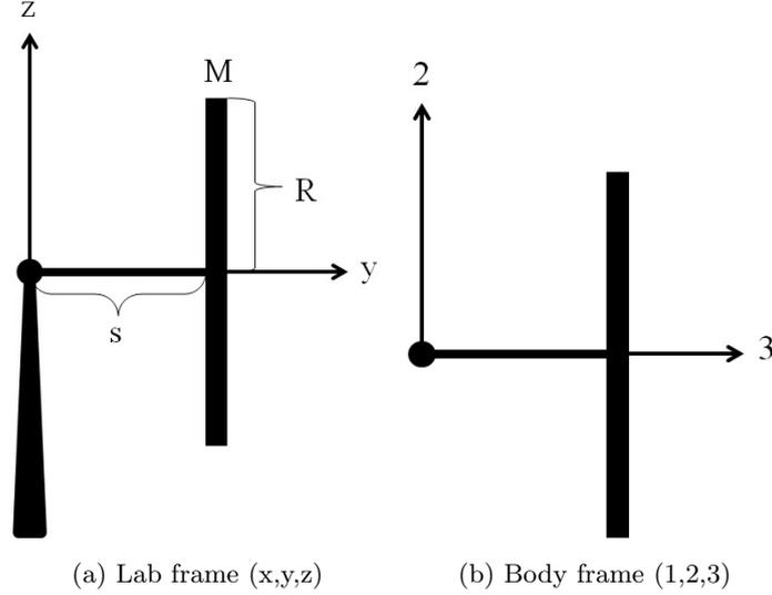
Figure 3: Setup of the experiment with labeled dimensions and axes in both the lab (fixed) and body (rotating) reference frames
