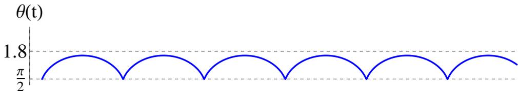
Figure 10: The point of the gyroscope traces out a cycloid as it precesses
